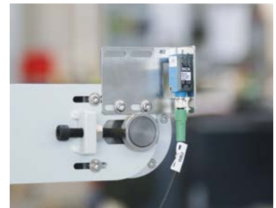
Photoelectric beam on the incoming belt side
