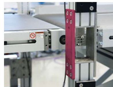
Easy belt replacement by dismantling a carrier element
