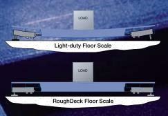
The exaggerated figure illustrates the problems of deck and load cell deflection. The RoughDeck design minimizes deflection of the deck and feet.
